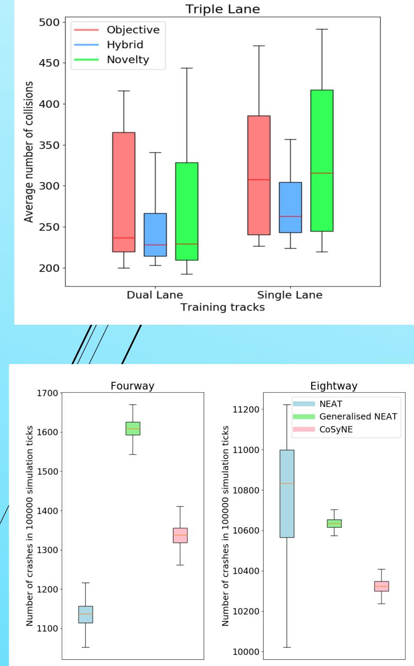
The results (right) indicate that the coevolved techniques outperform generalized systems. In the simplest case of the four-way intersection, this difference is quite extreme, but in the more complex example of the eight-way the difference is much smaller.
